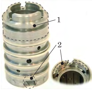
Figure 5.10 Design of the valve body including the crown, 1, and the inclined groove, 2. The crown is glued to the original valve body and secured with the help of pins.
