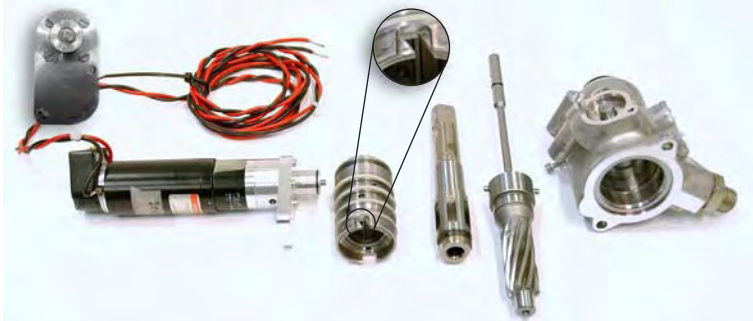
Figure 5.9 Photo of the mechanical design of the Active Pinion. Seen in the picture from the left are the DC-motor including the excenter, the valve body with the inclined groove, the spool, the pinion including the torsion bar and the pin guiding the valve body and finally the housing of the valve. This is prototype IV.
