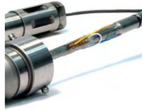
Figure 5.11 Full bridge contains four strain gages, which have been mounted on the torsion bar. The wires exit in two drilled holes in the top of the torsion bar.
