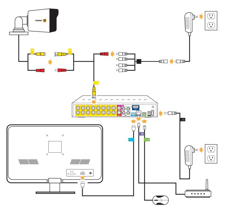
Monitor/TV not included. Connections applicable to all 4, 8, and 16 channel models. Connections may vary by model Please ensure the DVR is connected to a monitor/TV and that you have chosen a password on your DVR before proceeding Please ensure the monitor/TV is powered off when connecting DVR.
